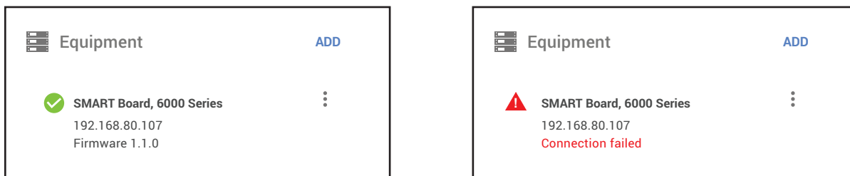
Figure 5: When Mira Connect can communicate with the device, a green check mark is visible, otherwise a red triangle indicates Mira Connect could not successfully communicate with the device.
