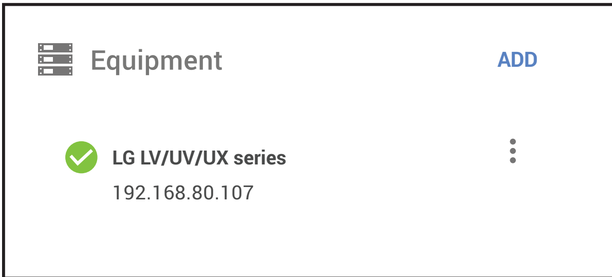
Figure 4: When Mira Connect can communicate with the device, a green check mark is visible.
